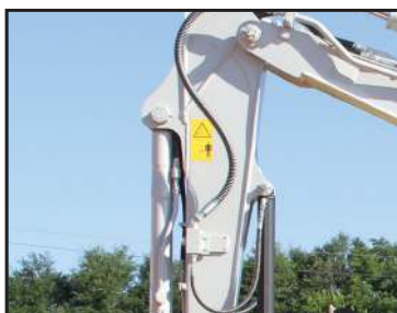
Auxiliary Hydraulic Lines
